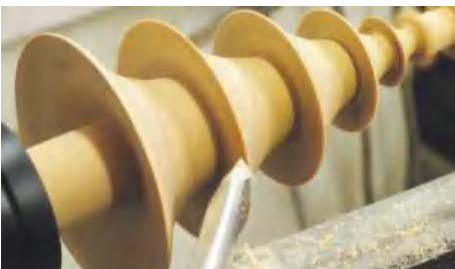
▲ Pic.9 Using the gouge in a bevel rubbing cut will give a good finish. First, check the tool will fit easily in the place where you want it to go
